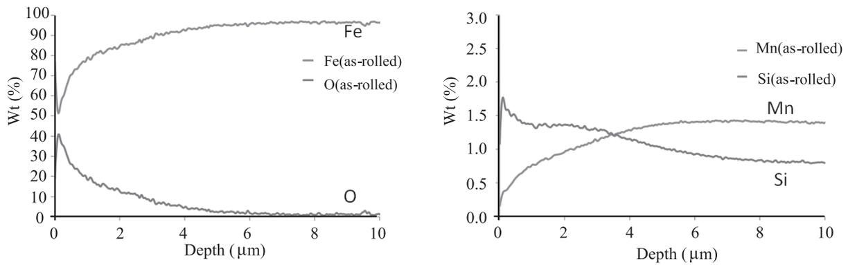
Fig.3. GDOES depth profiles for (a) Fe-O and (b) Si-Mn analyses of the as-rolled sheet containing rolled-in scale.
