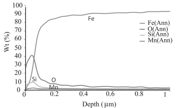
Fig.5. GDOES depth profiles of the annealed sheet containing rolled-in scale.
