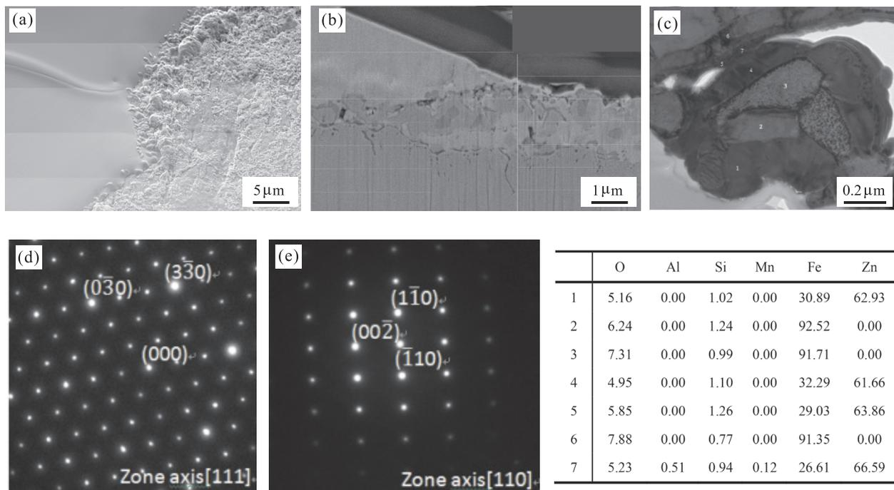
Fig.8. Cross sectional analysis of galvanized sample by TEM/EDS and SAED.
