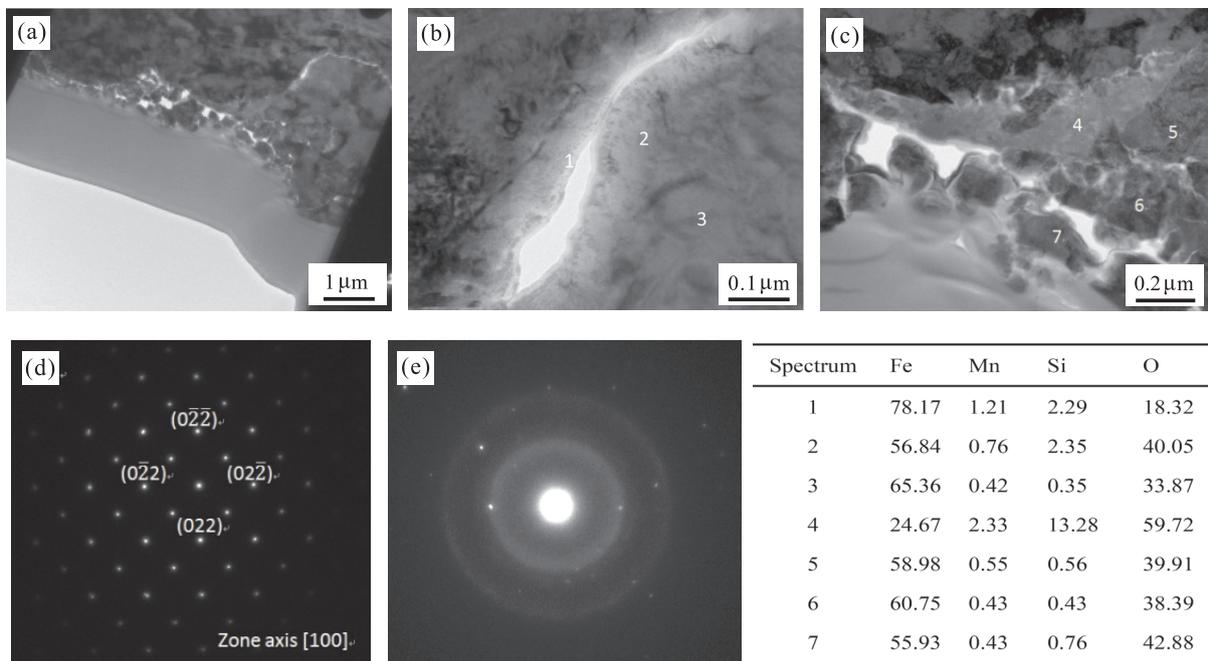
Fig.4. A series of TEM analyses of the cross section of the hot-rolled-in scale area.
