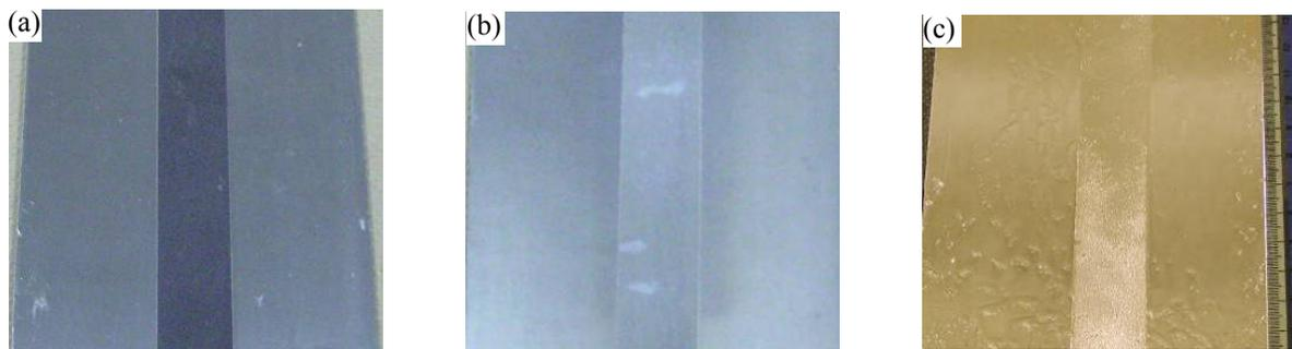
**Fig.2.** Images of the (a) as-rolled, (b) annealed and (c) galvanized, Mn/Si DP steel samples.
