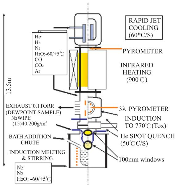
**Fig.1.** Schematic diagram of the galvanizing simulator.
