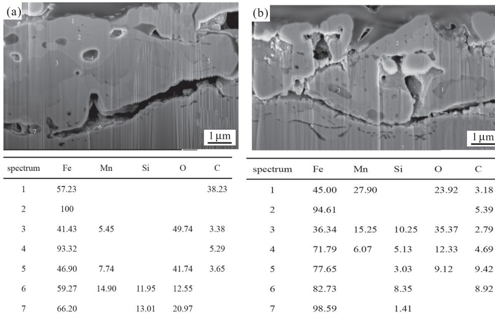
Fig.6. Cross sectional analysis of SEM/EDS in the rolled-in scale area of the annealed sample.
